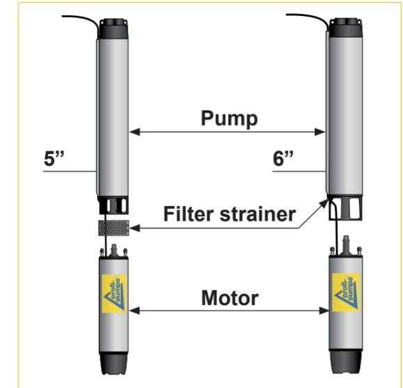
**The filter strainer of the 6-inch pump is already installed in the pump component (visible around the pump shaft).**
