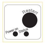
1. The green light when on indicates that power is on. The red light when on indicates that the pump is off due to either a fault present, pipeline failures and other pipeline water conditions. Open a faucet at the end of the installation as shown. When power is switched on, the green light turns on and the pump starts running. A few seconds later, water pipes should have water running through them. If there is no water coming out of taps, stop the pump and press the "Restart" button.
