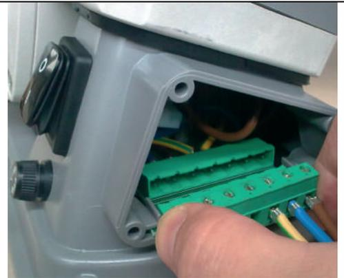
Insert the connector and close the side cover.
