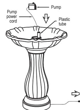
5.3 Place upper reservoir onto lower column and twist the upper reservoir clockwise to secure.
