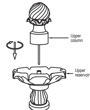
5.5 Attach pump to the rubber hose. Then place the upper fountain body into lower reservoir and twist the upper fountain body clockwise to secure.
