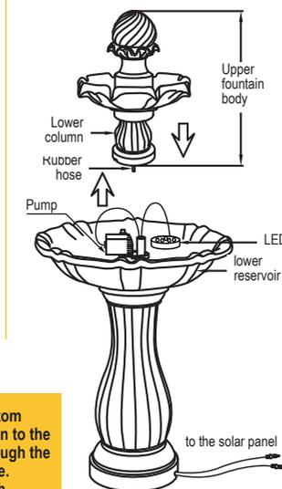
5.6 Fill reservoir with appropriate amount of water to completely submerge the pump.
