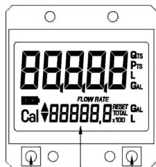
RESET button LCD Display CAL button
