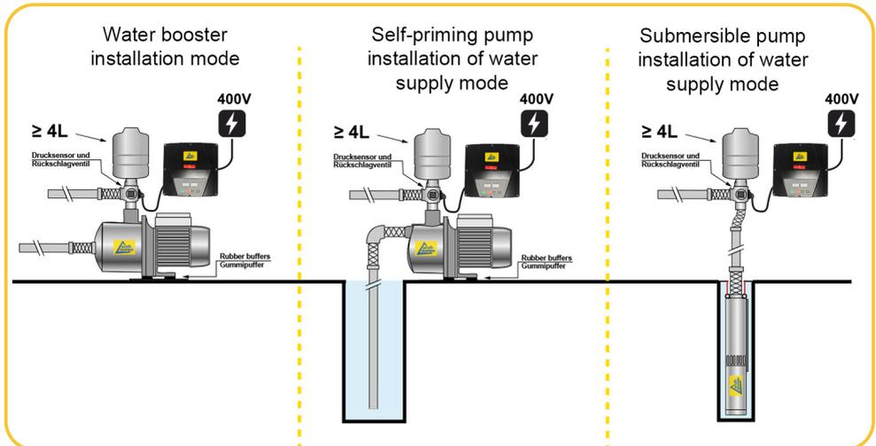
A non-return valve on the discharge side of the pump is absolutely necessary. We recommend the installation of a 5-way adapter with built-in non-return valve from our product range, which is available to suit the line cross-section. These 5-way adapters have the possibility of connection for the pressure sensor\*, as well as for an additional pressure gauge (special accessory, Art.-No. A7257, A7258, A7259, A7260, A7261)
