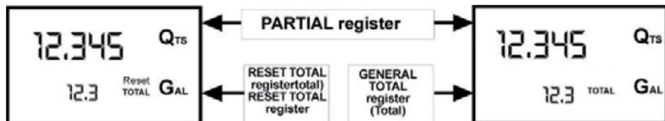
NOTE: 6 digits are available for Totals, plus two icons x 10 / x100. The increment sequence is the following: 0.0 > 99999.9 > 999999 > 100000 x 10 > 999999 x 10 > 100000 x 100 999999 x 100
